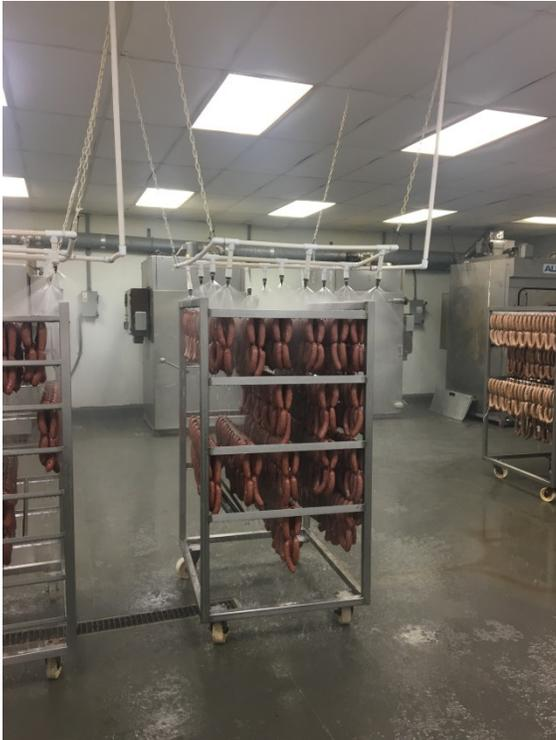
*Once the links have been made, they are sent to the oven to be baked. This is a picture of the links being cooled in a cold shower before heading to the freezer.*
